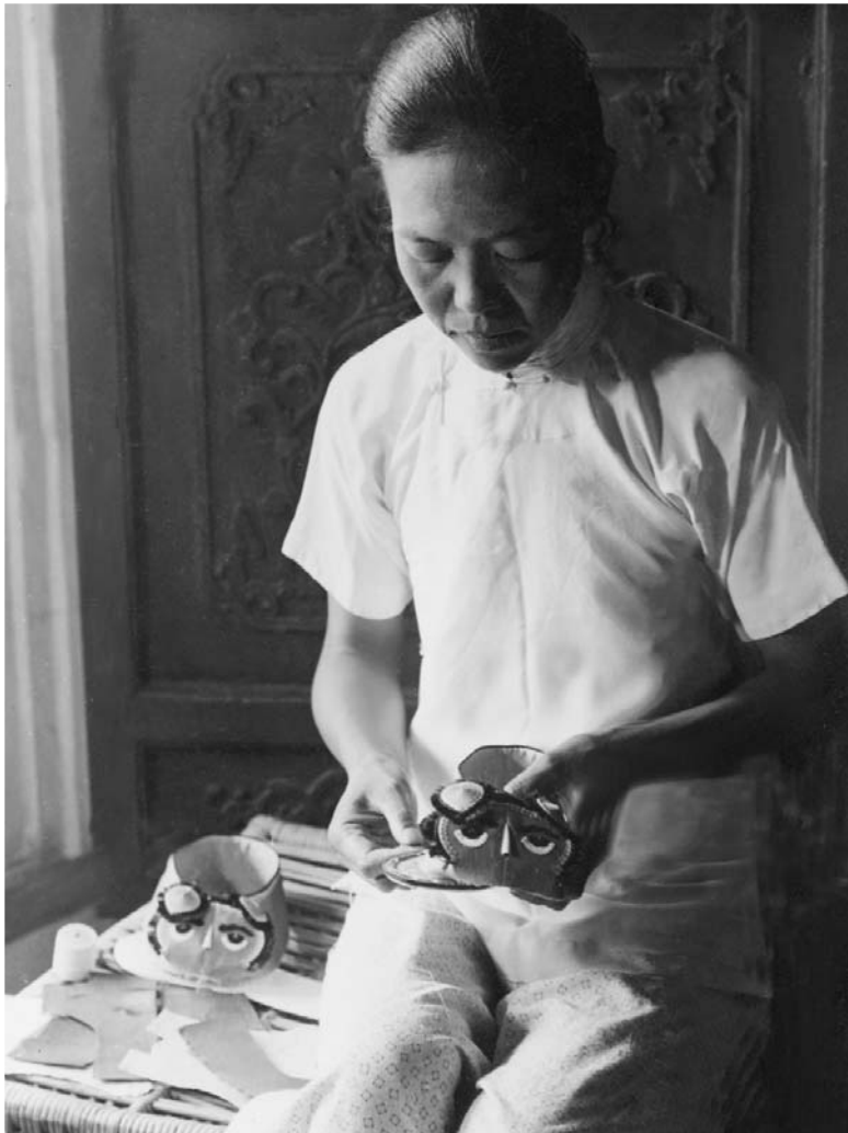
Clockwise: Fitting the sole to the upper of a child's shoe.
