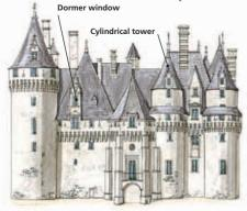
**Ussé** (see p101) was built in 1462 as a battlemented fortress. Later, the walls overlooking the main court-yard were modified during the Renaissance, with dormer windows and pilasters. In the 17th century the north wing was replaced by terraced gardens.
