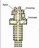
The plan of St-Benoîtsur-Loire is typical of Romanesque architecture, with its cross shape and rounded apse.
