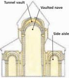
A section of La Collégiale de St-Aignan-sur-Cher shous Romanesque tunnel vaulting. The vaulted side aisles provide added support for the bigh nave.
