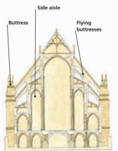
A section of St-Etienne in Bourges reveals its five divisions with two aisles on either side of the nave. The building also has five portals rather than the usual three.
